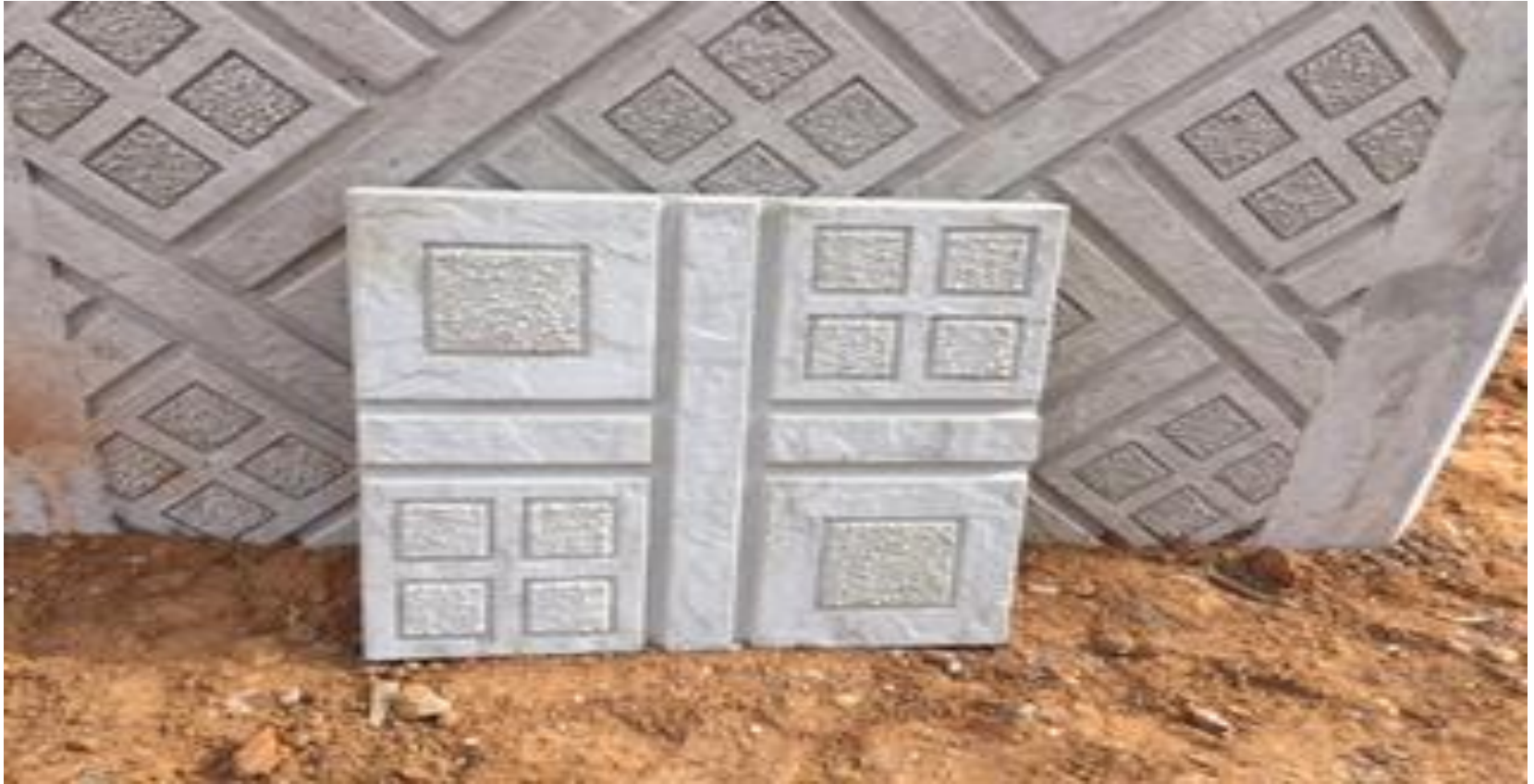
MSE Wall panel mock up
